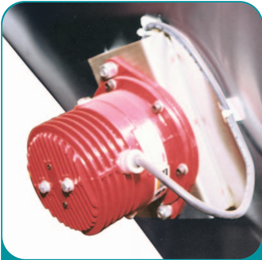
Syntron® model V-41 Electromagnetic Vibrator installed on a stainless steel bin.
