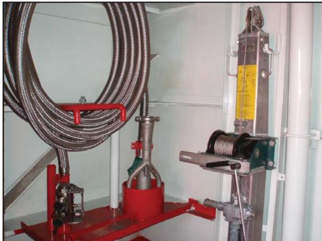
The pump and hoses must always be safely supported and fastened in order to avoid wear or damages due to ship movements. It is especially important that the hoses are not hanging or laying over sharp edges, or that sharp objects are placed upon them. The bending radius for the hoses during storage must not be less than specified.
