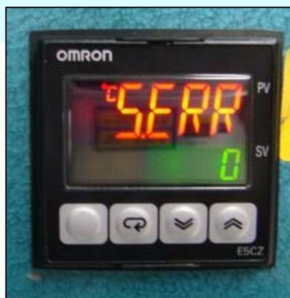
It could be a few things, the most common is the thermocouple is broken and needs changing.
