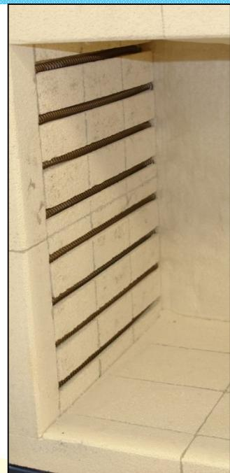
Take note of how they come out. This will help you to understand how to install the new elements into the grooves in the furnace. Once old elements are out, make sure to vacuum all grooves out as dust, parts of an old element and any other build up will shorten the life span of the new elements.
