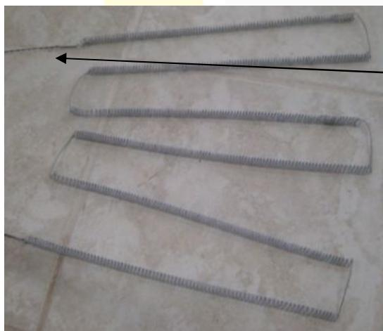
Lay new elements out and make sure they are not tangled. Pick up by the element tail and thread into the hole through the bricks and out the back of the furnace.
