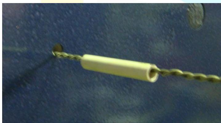
Slide ceramic tube back over the element tails top and bottom.
