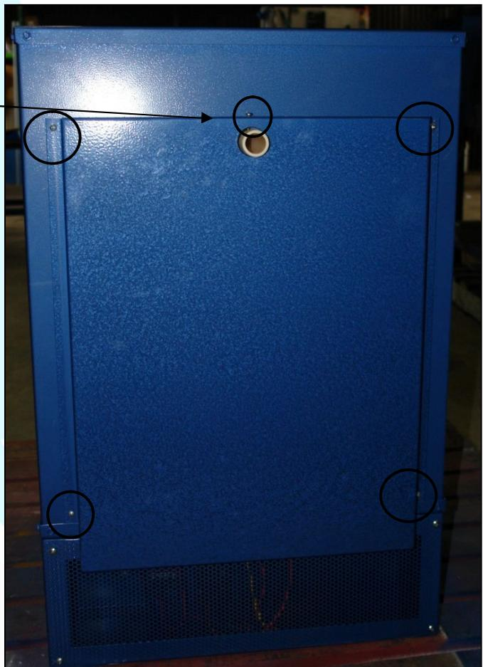
Then unscrew the four mounting bolts on the back panel.
