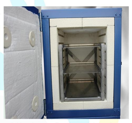
The door has a micro switch installed that will automatically cut power to the heating elements when the door is opened.
