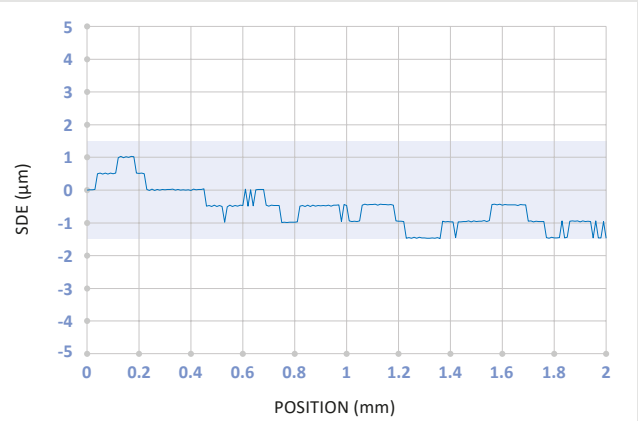
SDE (sub-division error) graph: accuracy of the interpolation device within the single pole pitch.
